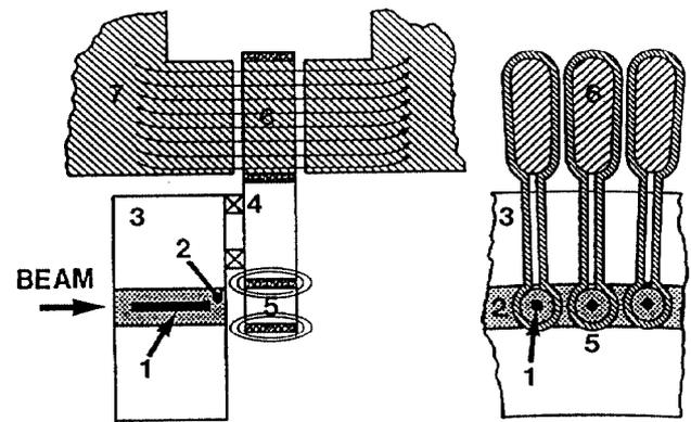
Fig.5: Radial cut and front view of the target wheel fitted with an array of focussing, single turn induction coils. 1:Target rod; 2:Graphite container; 3:Copper wheel; 4:Electrically insulating fixture; 5:Single coil solenoid; 6:Induction loop for solenoid; 7:Stationary, pulsed C-magnet.
