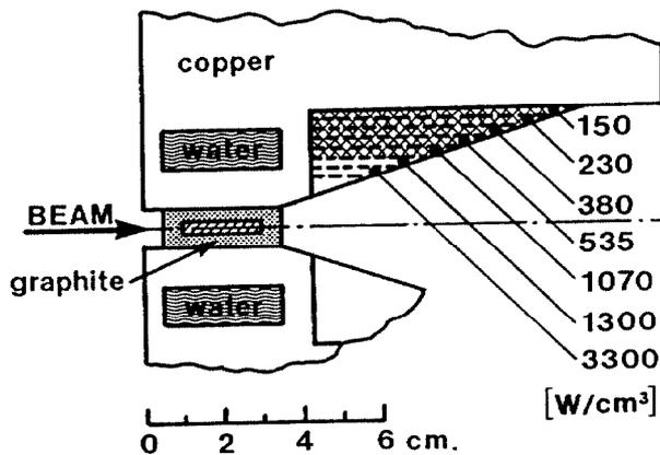
Fig.3: Radial cut through the periphery of the target wheel. The power densities in the dashed downstream zone are those for stationary copper, not rotating with the wheel.
