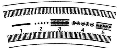
Fig.2:Various possibilities to mount the target material (solid parts) around the periphery of the water cooled target wheel. The target ribbon resp. rods are inserted either directly into the copper (1,2) or into intermediate graphite jackets (3,4,5).
