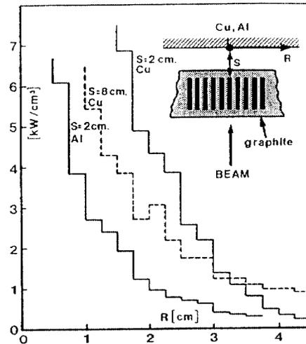
Fig.4: Power densities for stationary copper resp. aluminium placed downstream of the target wheel in the shadow of the graphite ribbon, containing the target rods.
