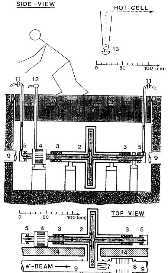
Fig.1: Side and top view of the  $e^+$ -target station. 1:Target Wheel; 2:Vacuum Tank; 3:Rotating Vacuum Feed-Through; 4:Motor; 5:Rotating Water Feed-through; 6:Tungsten Target; 7:Solenoid; 8:Acceleration Stage; 9:Beam Pipe; 10:Mobile Top Shield (Thickness 80 cm); 11:Cooling Water In/Outlets; 12:Electrical Supply; 13:Overhead Crane; 14:Local Shield.
