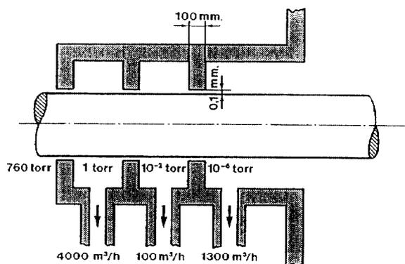
Fig.6: Feed-through for the rotating axis of the target wheel into the vacuum, achieved by differential pumping of a series of stationary chambers around the axis.
