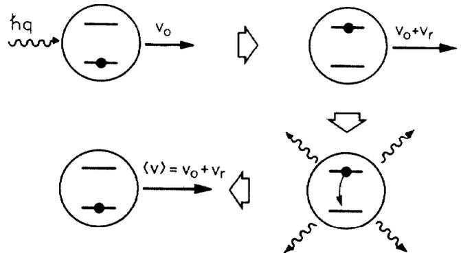
Fig. 3. Principle of laser cooling.
