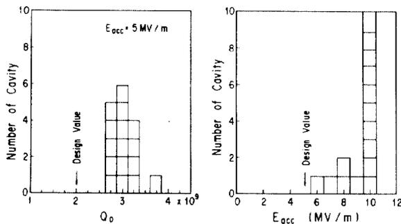
Fig. 6 Maximum accelerating fields, E<sub>acc</sub>, and Q-values at E<sub>acc</sub> = 5 MV/m of the 16 five-cell superconducting cavities tested in a vertical cryostat.
