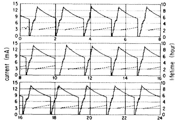
Fig. 3 Total beam current (solid line) and beam life time (dotted line) in the TRISTAN-MR recorded through 24 hours on February 28, 1988.
