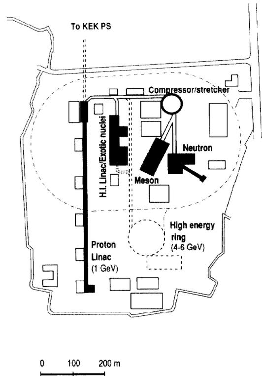
Fig. 11 Accelerator layout of the Japanese Hadron Facility.
