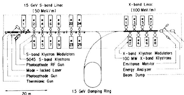
Fig. 9 Test Accelerator Facility for the linear collider R&D at KEK.
