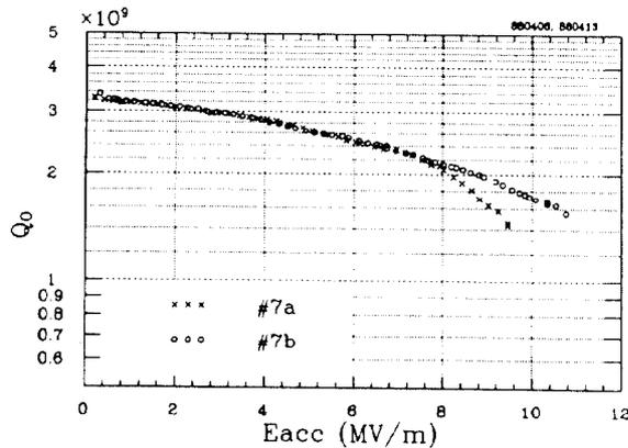
Fig. 5 Q-values of the two five-cell superconducting cavities as a function of the accelerating fields, E<sub>acc</sub>.
