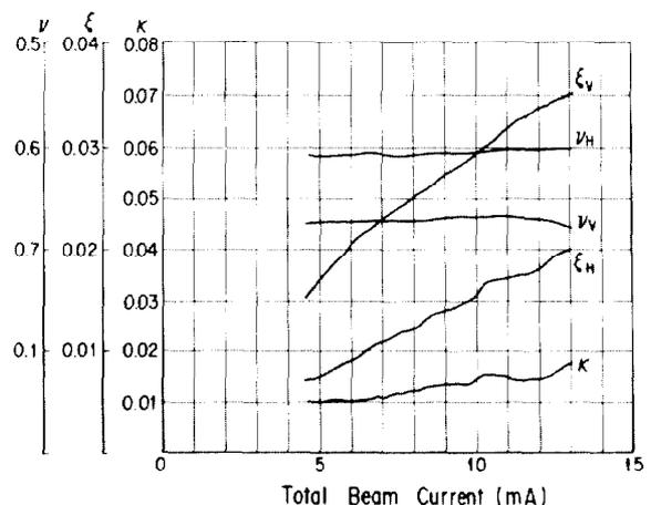
Fig. 4 Horizontal and vertical betatron tunes,  $\nu_H$ ,  $\nu_V$ , beam-beam parameters,  $\xi_H$ ,  $\xi_V$ , and vertical to horizontal emittance ratio,  $\kappa$ , as a function of the total beam current in beam collision at 28 GeV.
