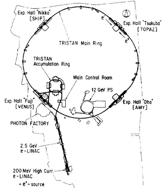
Fig. 1 Site layout of the TRISTAN accelerator complex.
