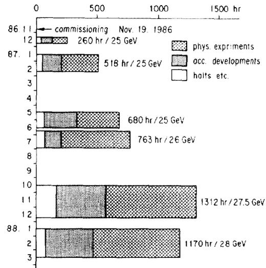
Fig. 2 Summary of the TRISTAN accelerator operation after the beam commissioning in November 1986.
