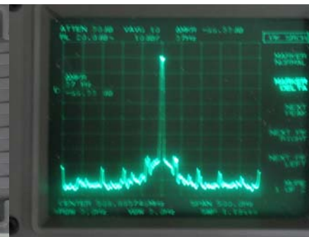
Span 500 Hz Sideband peaks at 32, 37, 46, 50, 100 Hz.
