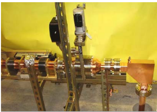
The uncompressed arm has a variable phase shifter and a gate valve
