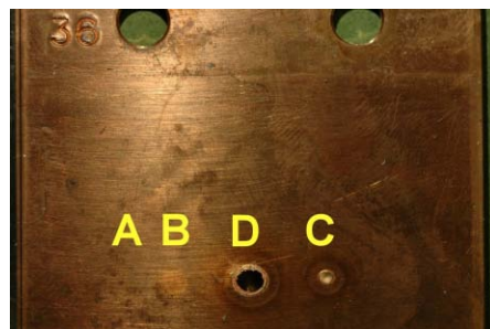
Figure 2: Impact of a 450 GeV/c beam from the CERN SPS onto a Copper plate inserted into a 20 cm long target [2]. The position of this plate within the target corresponds approximately to the peak energy density. Four beams of different intensities were sent to the target: 1.2 \times 10^{12} (A), 2.4 \times 10^{12} (B), 4.8 \times 10^{12} (C) and 7.2 \times 10^{12} (D) protons.
