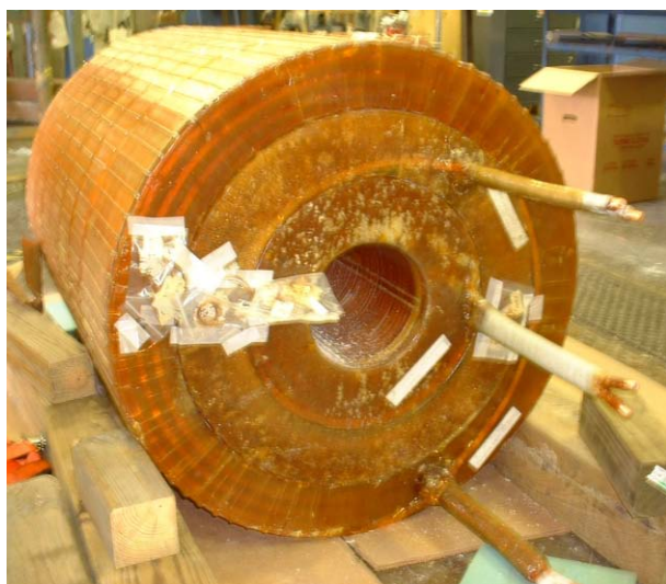
Figure 6: The nested set of 3 coil segments. The axial and circumferential grooves are visible on the outer surface of the coil.
