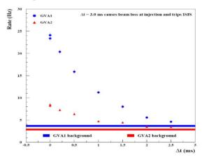
Figure 5: Rates of proton counts in scintillation counters GVA1 (circles) and GVA2 (triangles) placed in the MICE beam-line, plotted as a function of target delay,  $\Delta t$ , for a constant dip depth after the optimum insertion time. The one-standard-deviation background rate bands are shown for GVA1 (upper band), and GVA2 (lower band).
