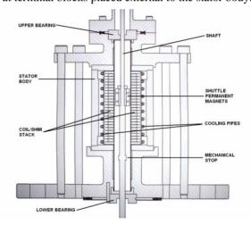
Figure 1: The stator mounted in its supporting flanges. The stator body with its end caps measures 90mm. (Note that the full length of the target shaft [560mm] and the optical readout block are not illustrated.)
