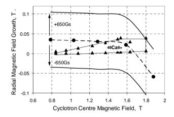
Figure 2: The working diagram area (triangle) and the real magnetic field behaviour (line with circles) of the U400R cyclotron.
