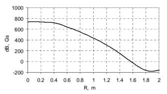
Figure 4: The sum contribution of the ten radial trim coils at the average magnetic field level 1.8T.
