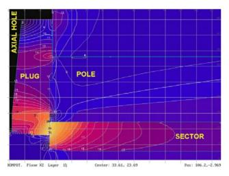
Figure 6: Magnetic field distribution in the vertical section of the magnet centre region with the small diameter of plug axial hole.
