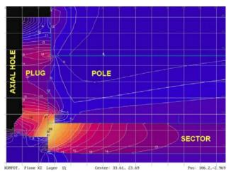
Figure 7: Magnetic field distribution in the vertical section of the magnet centre region with the big diameter of plug axial hole.
