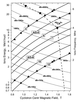
Figure 1: The working diagram of the U400R cyclotron.
