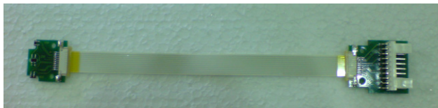
Figure 4: flexible hall probe design
