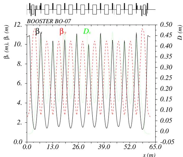
Figure 1: Booster arc: beta and dispersion functions for the nominal lattice.
