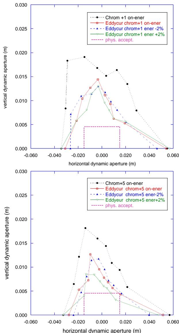
Figure 3: Dynamic apertures at the injection point at  $200$  MeV, where the eddy current effect is strongest, calculated for 1028 turns with chromaticity  $\xi_x, \xi_y = (+1, +1)$  (top) and  $\xi_x, \xi_y = (+5, +5)$  (bottom).
