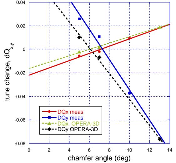
Figure 2: Tune changes as a function of the horizontal end chamfer angle in the short dipoles. Data points calculated, both from simulations (OPERA-3D) and measurements on the pre-series, with different chamfer cuts, are compared. The chosen chamfer angle of  $7.5^\circ$  gives almost the nominal tunes.
