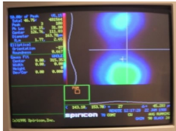
Fig. 2. Synchrotron light image kicking every other turn.
