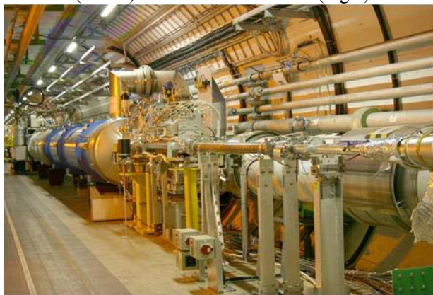
Figure 1: LSS picture showing a standalone cryomagnet and ambient vacuum sectors.
