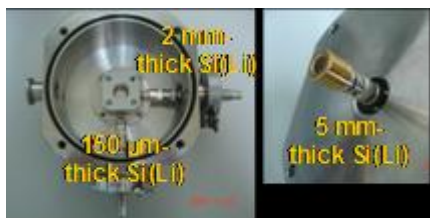
Figure 3: Photograph of the experimental set-up and detectors installed inside detector chamber.
