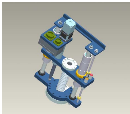
Figure 1: Electric Cylinder Powered Actuator Developed for the SNS MEBT Diagnostics Chamber
