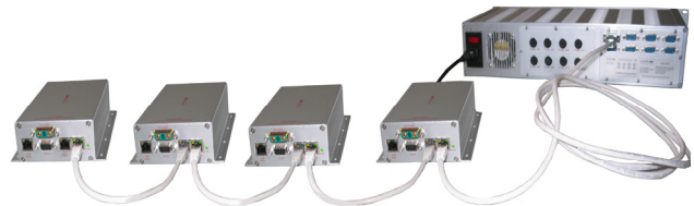
Figure 1: BSC modules connected in a daisy chain and connected to a microIOC-CosyIcon as the central processing unit. To each BSC to Bergoz detectors can be connected (not shown).
