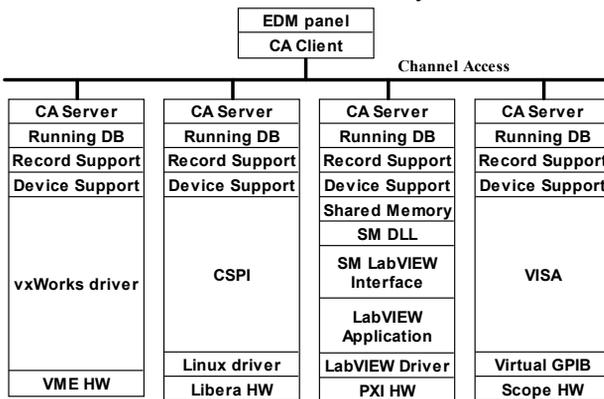
Figure 2: Diagram of SSRF BI software system
