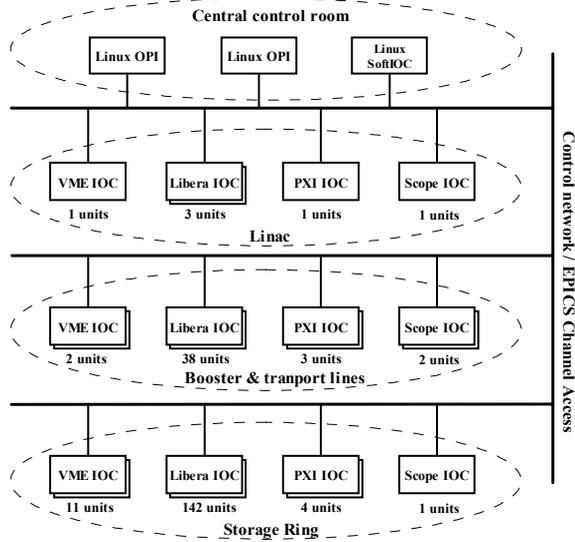
Figure 1: SSRF BI data acquisition system architecture
