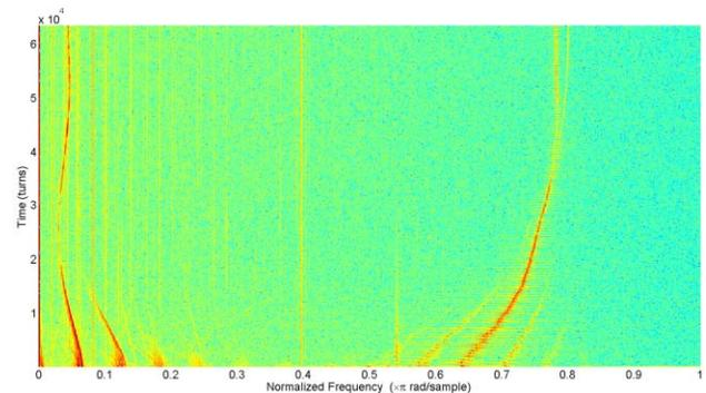
Figure 3: Ramping tune measurement in the booster
