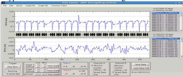
Figure 4: Measured COD in the ring
