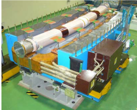
Figure 5: Ceramics vacuum chamber installed in BM
