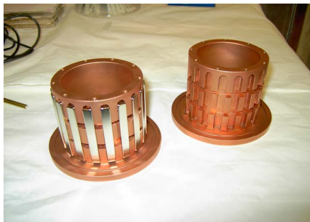
Figure 7: Plasma chamber magnets in multicusp arrangement.
