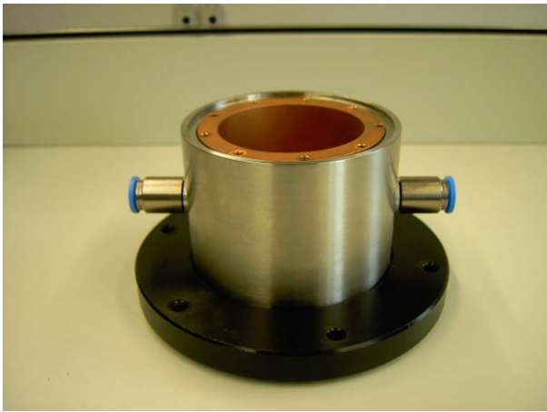
Figure 8: Plasma chamber with a water cooling coating.
