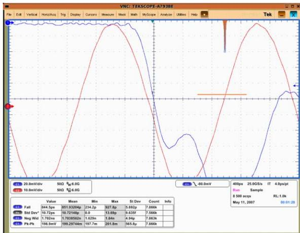
Figure 4: The jitter of WCM output.
