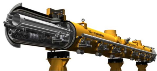
Fig. 2. A view of a cryomodule with cavity-string installed.
