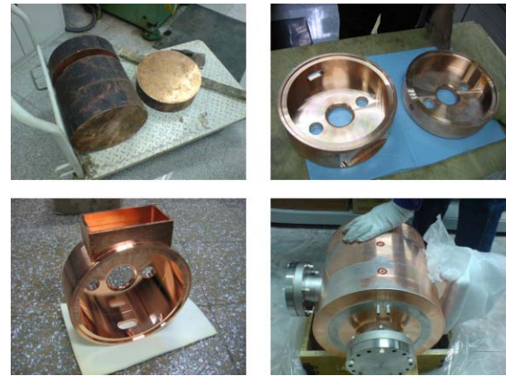
Figure 5: Pictures of different period during fabrication. (1) RAW material, (2) cells, (3) middle cell brazed with waveguide, (4) hole brazed cavity
