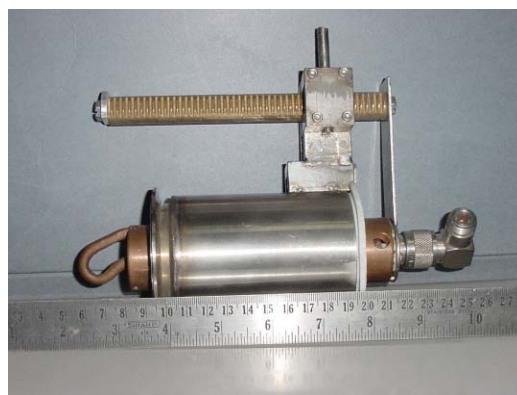
Figure 3. Picture of the drive coupler to feed power
