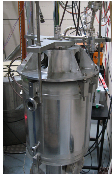
Figure 1: Cavity with helium tank and stiffening tube
