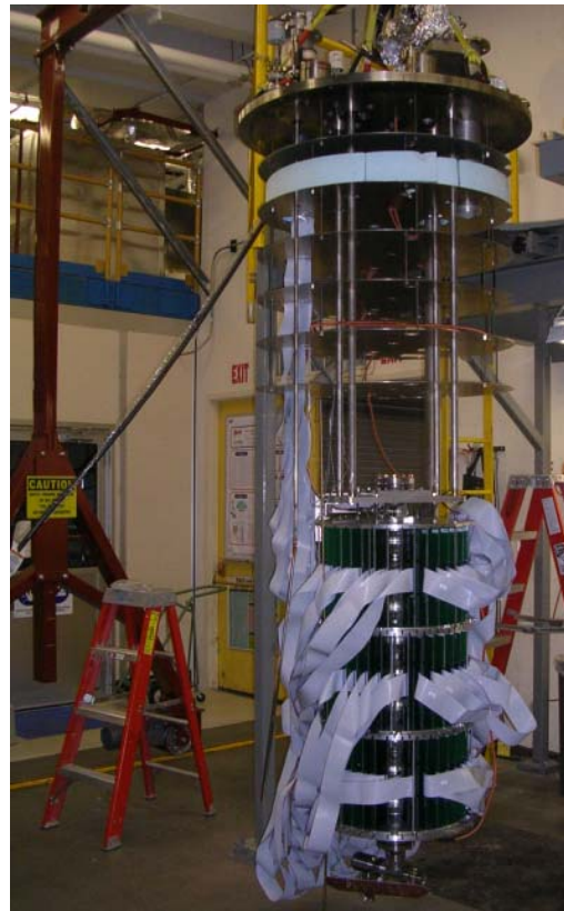
Figure 5: Cryostat insert showing the T-mapping boards along with connecting cables.
