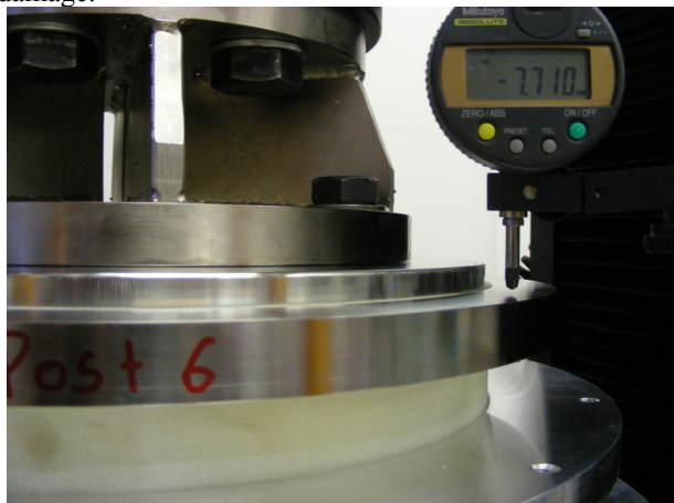
Figure 5: onset of failure: the upper disk is being dragged out of the fibreglass pipe.
