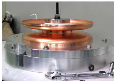
(b). Press a half-cell and decrease its TM010 \pi mode frequency.
