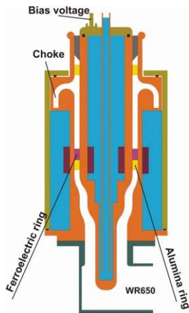
Figure 1: Coaxial ferroelectric phase shifter.
