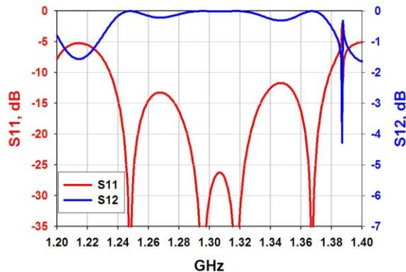
Figure 4: Frequency response of the new planar phase shifter.
