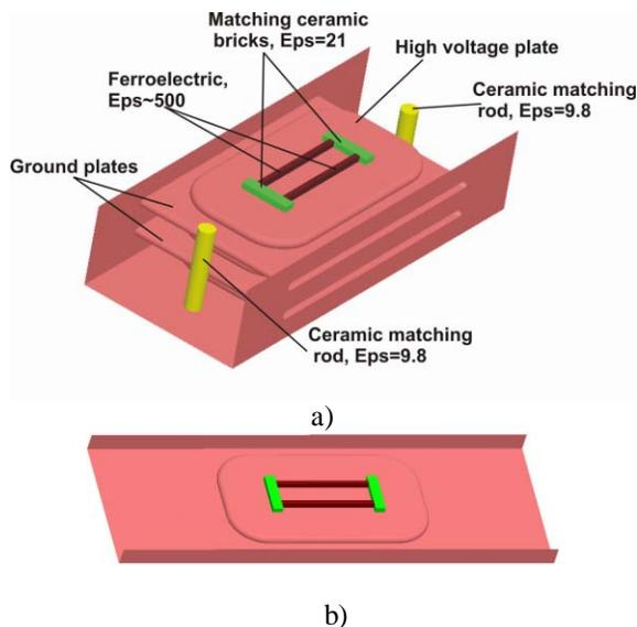
Figure 6: (a) Full: geometry of the three-layer phase shifter (top waveguide wall is removed); and (b) the assembly scheme of each layer containing two ferroelectric waveguides and two matching bricks.
