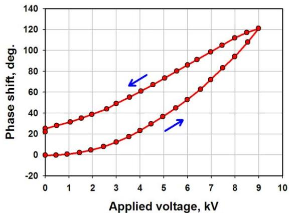
Figure 12: Phase shift versus bias voltage at 1300 MHz.
