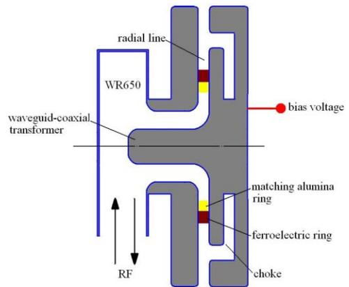
Figure 2: Coaxial-planar ferroelectric phase shifter.
