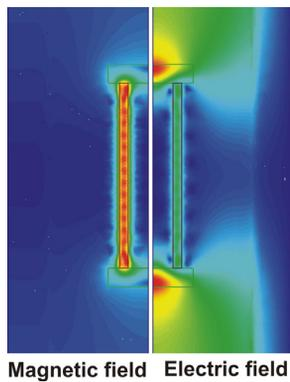
Figure 5: Field distribution in the phase shifter.
