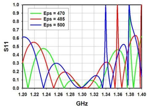
Figure 8: Calculated passband of the whole phase shifter.
