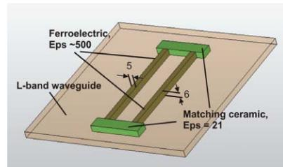
Figure 3: The new design of the planar phase shifter.
