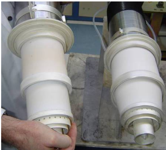
Figure 4: Standard tube (left) vs. new 90kW tube
