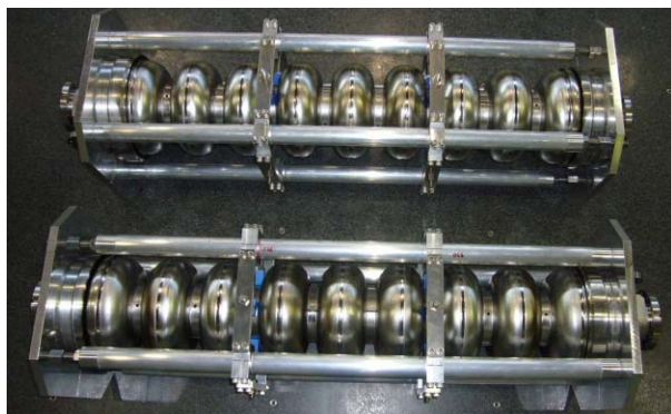
Figure 3: The STF 1.5-type cavities with transport jig
