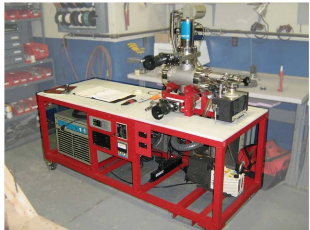
Figure 8 : Vacuum Test System.
