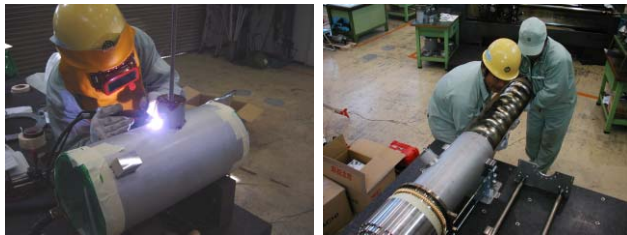
(a) Welding of Helium Jacket (b) Cavity Insertion to Jacket Figure 8 Assembly of a Cavity Unit
