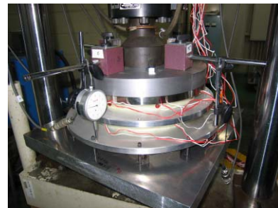
Figure 6 Loading Test of Support Post
