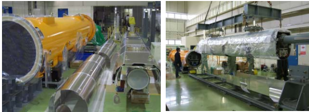
(a) Components of Cryostat (b) Assembly of Cryostat Figure 3 Components and Assembly of STF Cryostat
