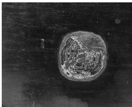
Figure 4: Fe Target surface after 30 minutes laser irradiation with 5 Hz. Laser power density and spot size was 2.4 \times 10^{-4} \text{ W / cm}^2 and 7.6 mm, respectively.
