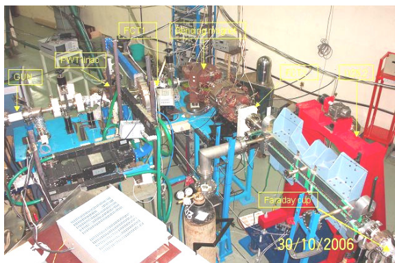
Figure 7: Beam transport line for acceleration trials.
