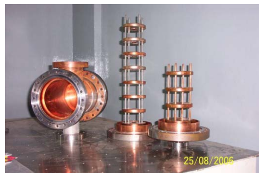
Figure 3: Photograph of different components of 4 and 8 cell PWT structures.
