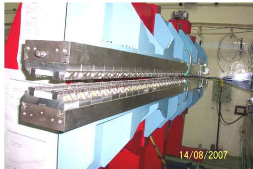
Figure 6: The two sections of the undulator. The corrector coil can be seen on the far end.
