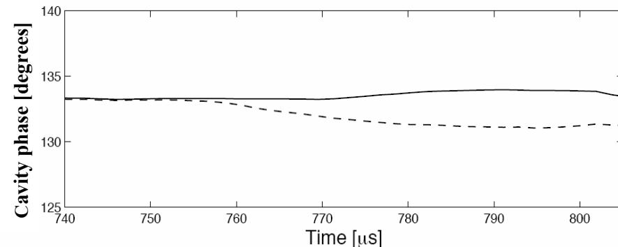
Figure 10: Cavity amplitude/phase under beam loading with (solid line) & without (dashed) AFF.
