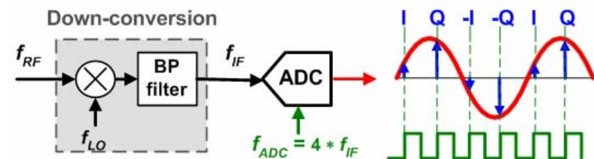
Figure 6: I/Q sampling scheme.
