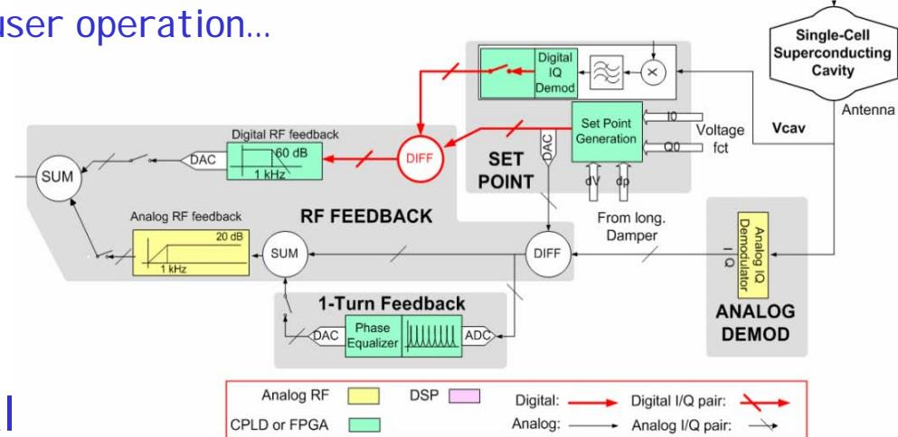
Figure 1: LHC RF Feedback loop
