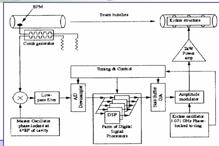
Figure 2: Bunch-by-bunch longitudinal feedback system for PEP-II.
