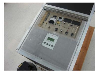
Three control cables and RF coax cable connect the two units. Total AC input power is 2 kW at 220 Volts.
