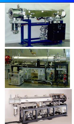
Linac Injectors of Synchrotrons for Therapy and Research
