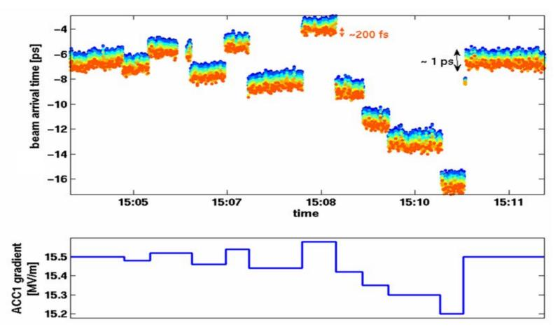
Time change seen by arrival time monitor:  $\sim 5 \text{ ps} / (\% \text{ ACC1 gradient change})$ Time change seen by TCAV:  $\sim 5.8 \text{ ps} / (\% \text{ ACC1 gradient change})$ Intra-bunch train jitter between two adjacent bunches:  $\sim 40 - 60 \text{ fs}$
