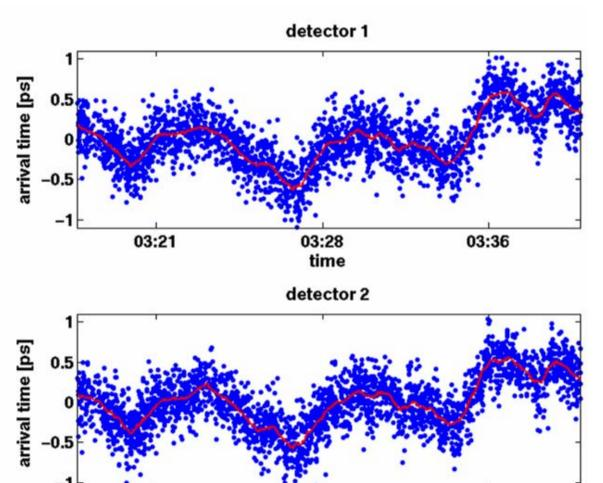
03:28 time The signal of the beam pick-up was split and connected to the two EOM detectors.
