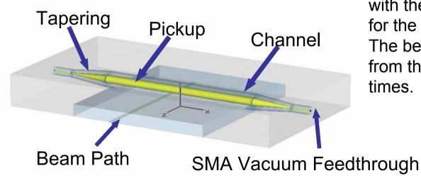
The arrival time of the pickup signals at both ends is measured with the same technique as used for the beam arrival time monitor. The beam position is determined from the difference of both arrival times.
