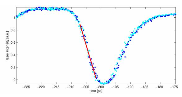
The resolution can be estimated from the slope of the phase monitor signal and the amplitude noise on the not modulated laser pulses:
