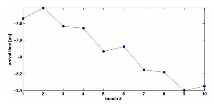
250 kHz oscillation of arrival time visible. (intermediate frequency of down-converters for cavity RF regulation)
