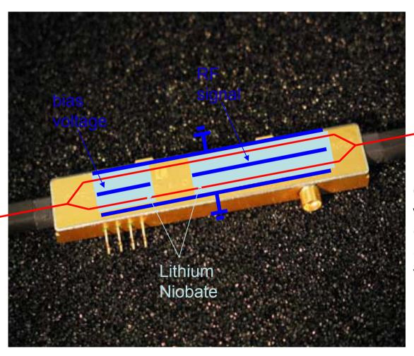
Commercially available with bandwidths up to 40 GHz (we use a 12 GHz version)
