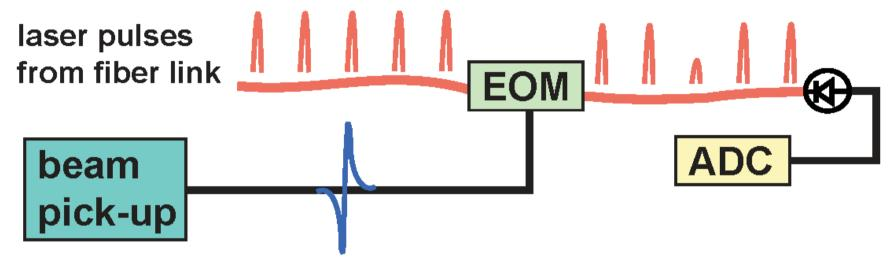
The timing information of the electron bunch is transferred into an amplitude modulation. This modulation is measured with a photo detector and sampled by a fast ADC.
