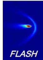
The beam is over-compressed in a way that the bunch length inside the chicane is short but long afterwards.
