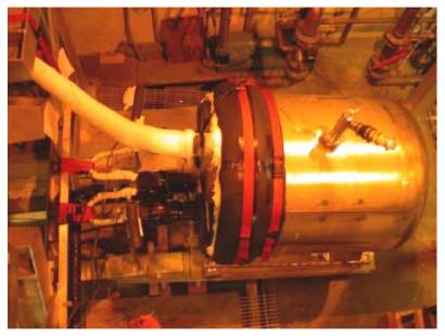
15-T solenoid during tests at MIT
