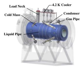
Figure 2: Magnet Cold Mass and Cryostat
