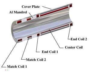
Figure 1: The Tracker Magnet Cold Mass Assembly
