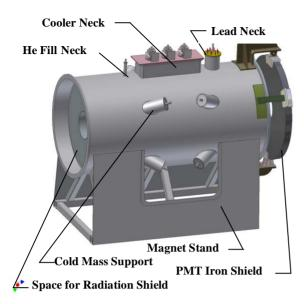
Figure 3: Tracker Magnet Vacuum Vessel
