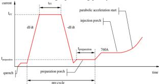
Figure 1: Parameters affecting decay during injection
