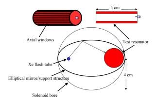
Figure 2: Sketch of the bench test system.
