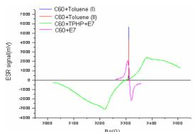
Figure 1: Comparison of time resolved (recorded at a fixed delay with respect to the laser pulse) EPR spectra for some of the test samples. Positive signal corresponds to absorption, negative to emission. 1G = 2.8 MHz; the position of the reference absorption peaks corresponds to 9.27 GHz [8].
