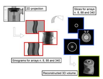
Figure 6: A schematic representation of the 3D image reconstruction procedure.
