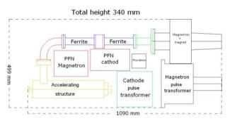
Figure 1: Design of a compact 5 MeV, S-band, 1 kW, electron linac for *in situ* applications.
