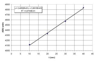
Figure 4: Grey level in ADU units *versus* exposure time showing the linearity of the imaging system.
