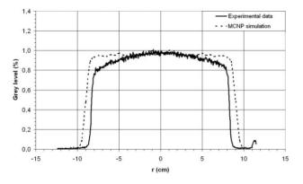
Figure 3: Comparison between the experimental x-ray spot profile and the MCNP simulation.
