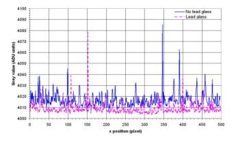
Figure 2: Area profile 1D projections showing the influence of lead glass on mottles reduction.
