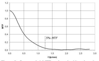
Figure 5: Pre-sampled MTF evaluated with a detection pixel size of 0.175 mm.
