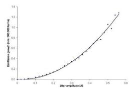
Figure 7: The simulated emittance growth due to a turn-toturn current-amplitude jitter for a wire length of 1m and a quadratic fit  $(4 * 10^{-9}I^2)$ .
