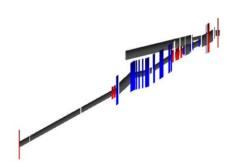
Figure 3: An example of BDSIM visualization - the 2 mrad ILC extraction line with photon and electron dump lines
