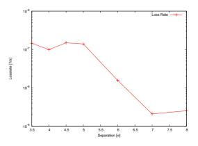
Figure 6: Loss rates vs beam separation with PLIBB.
