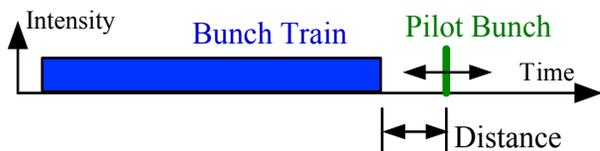
Figure 1: Schematic of a bunch train and a pilot bunch. We define the parameter, “Distance” or “D” as the bucket interval between the last bunch of a train and a pilot bunch.
