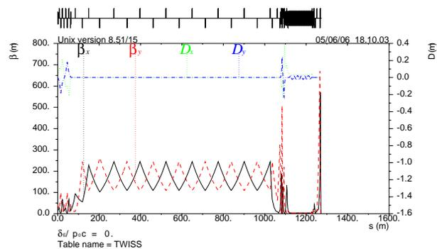
Figure 3:  $\beta$  functions and dispersion in SABER from the linac Sector-20 extraction point to the final focus IP.
