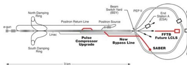
Figure 1: SABER at the SLAC accelerator facility.
