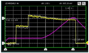
Fig. 4: Time evolution of the beam current (yellow) and the magnetic cycle (purple).
