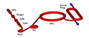
Figure 1: Schematic layout of the beta-beam complex.
