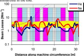
Figure 4: Loss distribution in terms of power deposition along one super cell of the PS machine for the case of <sup>6</sup>He (blue) and <sup>18</sup>Ne (red). The red and blue blocks indicate the position of the PS dipoles.
