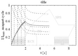
Figure 2: Cycle of the Beta-beam complex accelerating <sup>6</sup>He. For illustration purposes the single bunch intensities (dashed) are indicated for the 1st, 5th,10th, 15th and 20th bunch
